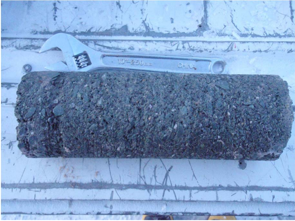
Photo 2: Drilled Core 8 (HB12-ND-CORE-DC8-QA-20120127) taken from 1+60 DS in the key trench.
