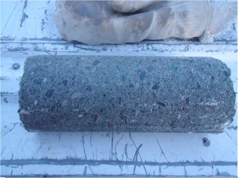
Photo 3: Drilled Core 9 (HB12-ND-CORE-DC9-QA-20120127) taken from 0+55 US in the key trench.
