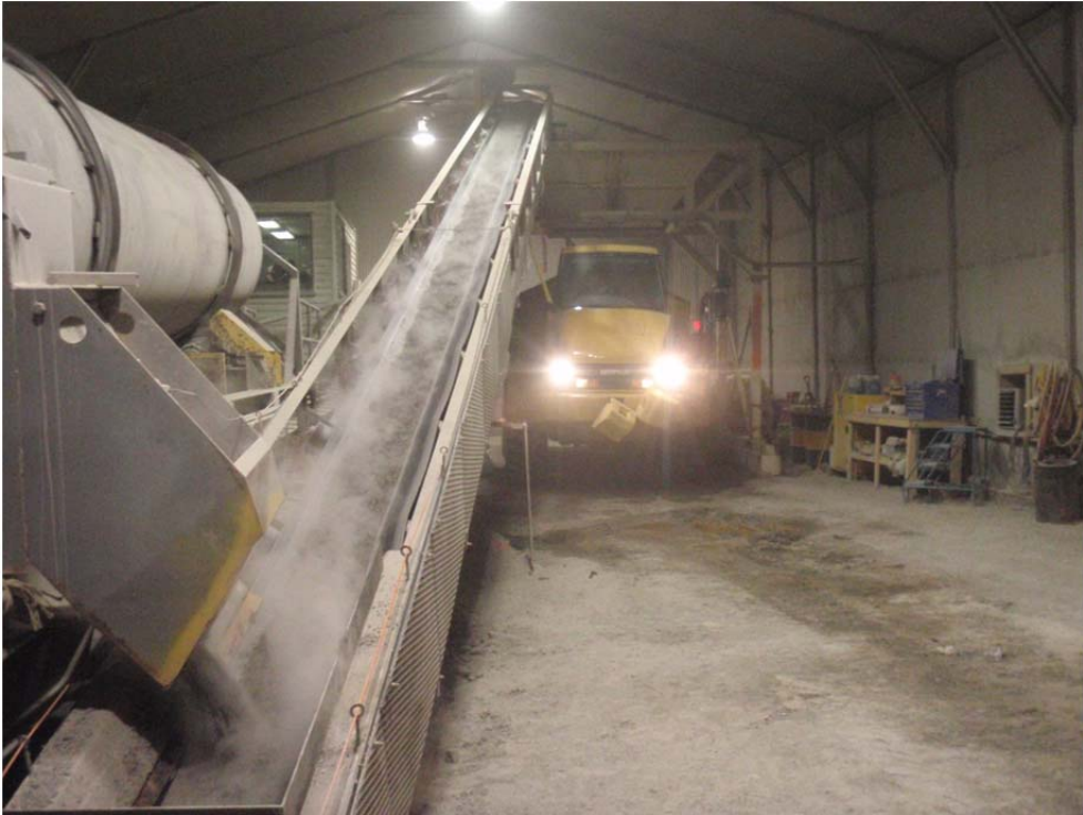
Photo 1: View of FCM exiting the FCP chute on dayshift. Note the steam coming off the now hotter (30+°C) material.
